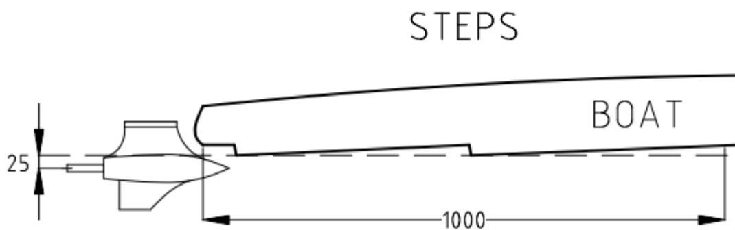
HYDROPLANE PROPELLER SHAFT HEIGHT MEASUREMENTS
