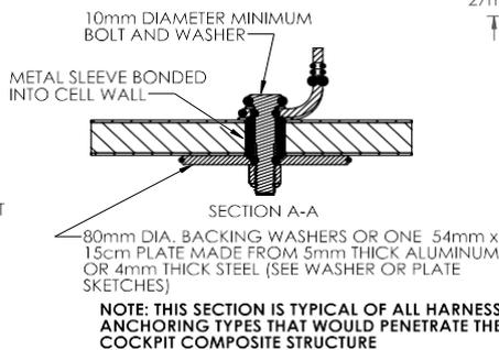
NOTE: THIS SECTION IS TYPICAL OF ALL HARNESS ANCHORING TYPES THAT WOULD PENETRATE THE COCKPIT COMPOSITE STRUCTURE
