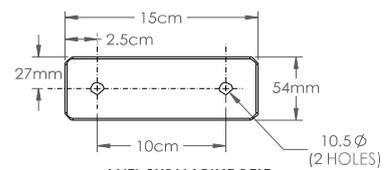
MOUNTING FASTENERS TO HAVE A MINIMUM TENSILE STRENGTH OF 150,000 PSI. AND BE CORROSION RESISTANT
